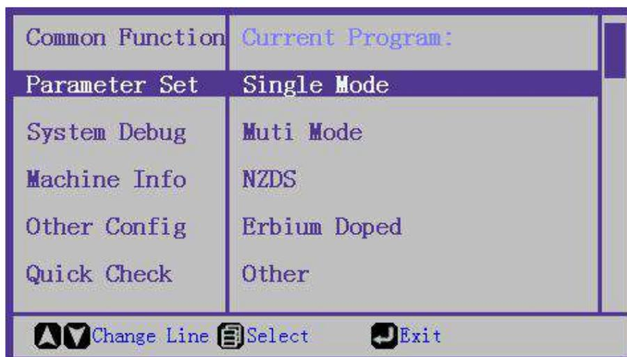
Press the “▲”“▼” choose the Procedure Number you need to operate or change, press the to choose the Procedure you want(the red is the current Procedure operating). If need to change the Procedure Parameters, please repress to enter the Procedure to change the detailed Parameters (DEFAULT is Factory settings, cannot be changed)
