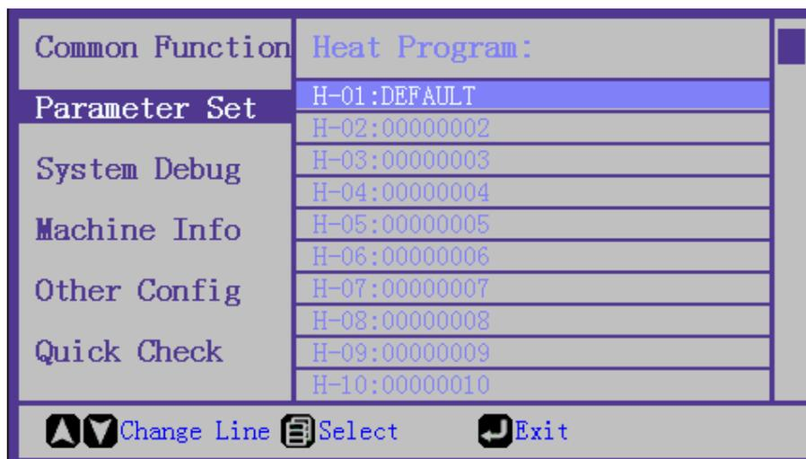
Press the “▲” “▼” choose the Procedure Number you need to operate or change, press the to choose the Procedure you want(the red is the Procedure operating now).If need to change the Procedure Parameters, please repress to enter the Procedure to change the detailed Parameters (DEFAULT is Factory settings, cannot be changed)
