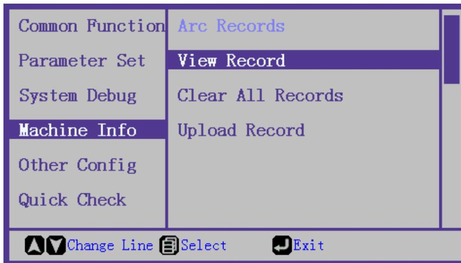
Enter “Arc times” menu by pressing and check arc records by pressing “◀”, “▶”
