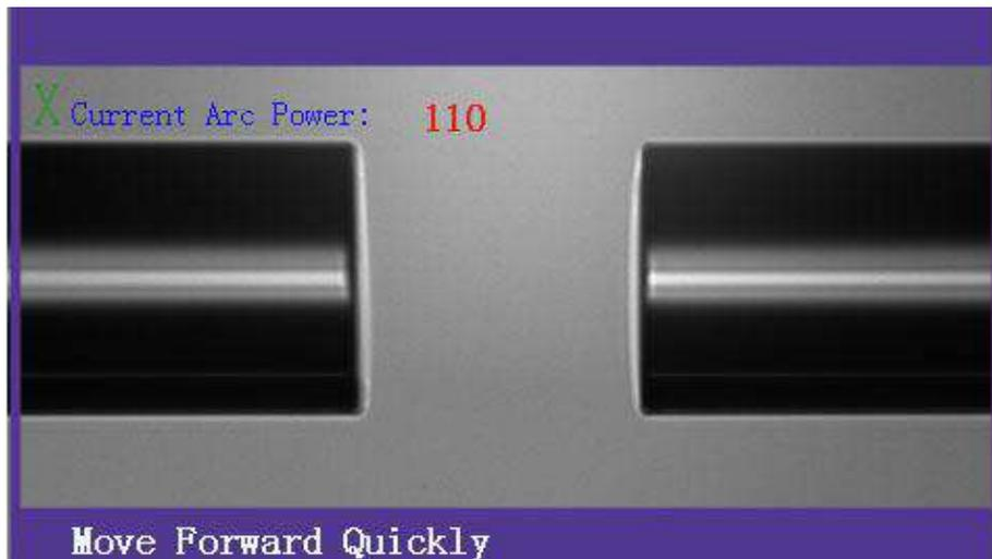
After arc, the screen shows a value, if the value is between 45-65, indicating the arc power is OK. If the value is less than 45, the arc power is weak, if the value is greater than 65, the arc power is too strong.
