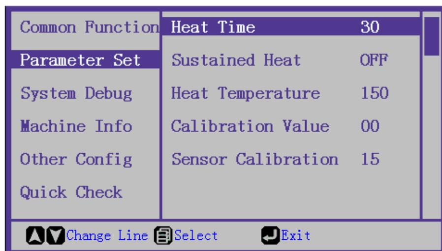
Press the “▲” “▼” to select, press the to enter the menu need to be changed, press “▲” “▼” change the detailed Parameters, then press the to save the result. When changing finished, press Exit.
